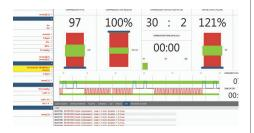
eCPR™ - Monitor CPR quality metrics in real-time including rate and compression depth, no-flow time, and excessive ventilation
