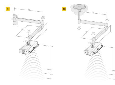
7 Double-joint wall arm, R1 = 480 mm, R2 = 480 mm, Wall arm swivelling ±90° and lockable, warmer rotatable 360°, vertical adjustment ± 45°
