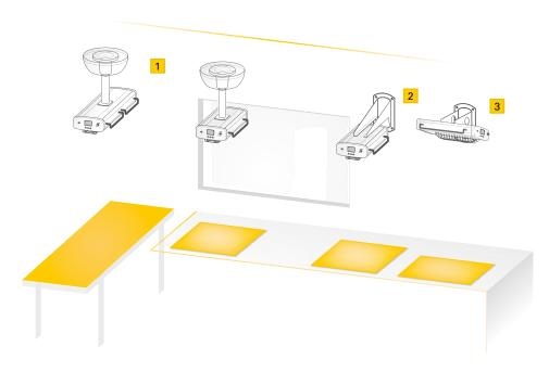
Ceiling bracket, distance between patient pad and bottom edge of solid ceiling max. 2600 mm
