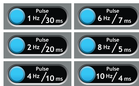
Select any PRF Pulse Width 2, 3, ... , 30 msec Select any PRF Pulse Rate 1, 2, ... , 10 Hz
